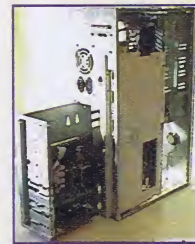
The EZPC-Tower system showing the A1200 and the PC motherboard (in slide-out frame)
